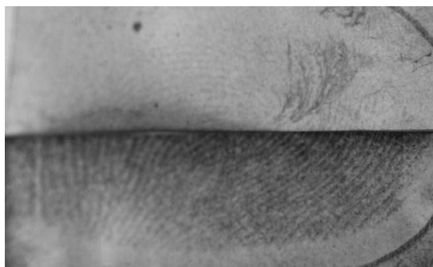
Fig. 1 Comparison between two halves of a sebaceous fingerprint on paper, developed by Ag-PD (top), and by Au-NP-C 18 followed by Ag-PD (bottom).
